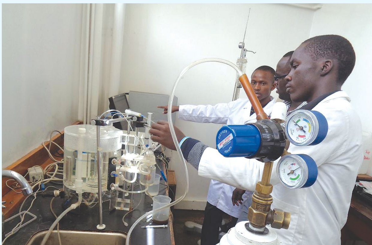
Medical Students carrying out an experiment using powerlab Langendorff apparatus with an isolated heart
